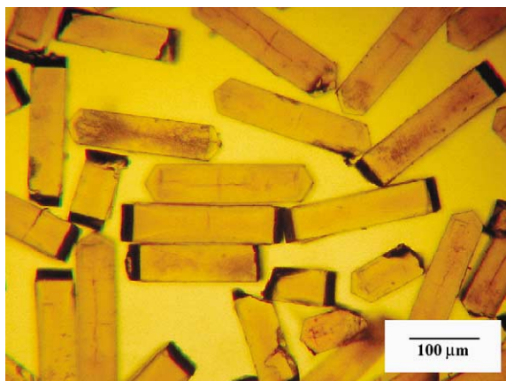
Fig. 10. Silicalite-1 crystals (sample 3) calcined in nitrogen in the cross-flow regime at T_{\text{max}} = 380^\circ\text{C} . Note that longitudinal and a transversal cracks exist in most crystals.
