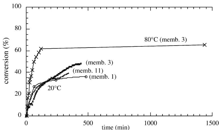
Fig. 3. Formic acid conversion as a function of time in a CMR at 20 and 80 °C. Please note the illustration of discrepancy shown for 20 °C by three similar membrane samples, obtained using the same preparation protocol.
