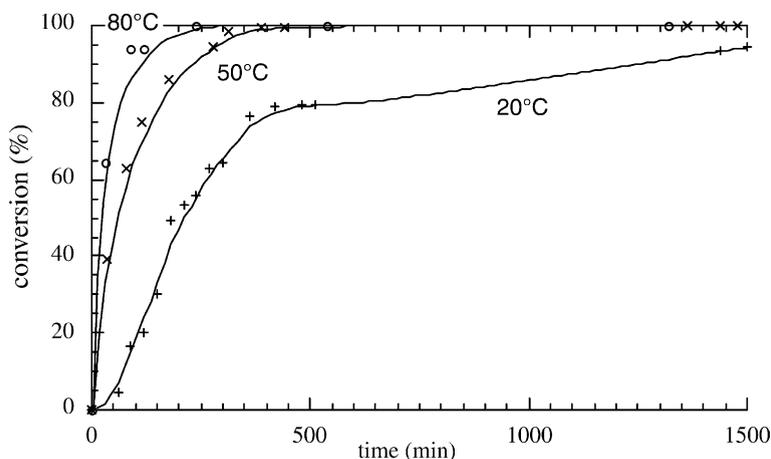
Fig. 2. Formic acid conversion as a function of time in a conventional, ideally stirred autoclave reactor at 20 (+), 50 (x) and 80 °C (o).
