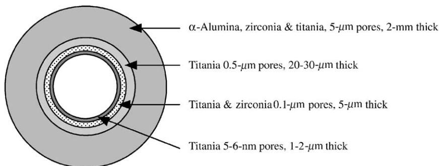
Fig. 1. Schematic cross-section of the membrane showing the four layers, their thickness and pore sizes.
