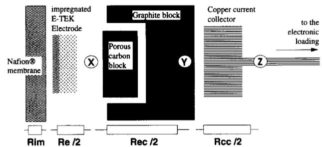
Fig. 3. Schematic drawing (half-cell) of the cell resistance components (X, Y, Z refer to potential measurement points).
