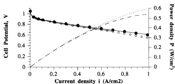
Fig. 4. Fuel cell potential–current density profiles (with power density) for Nafion<sup>®</sup> 117 EMAs with E-TEK ELAT electrodes loaded at 0.35 mg Pt/cm<sup>2</sup> under 4/6 bar pressure of H<sub>2</sub>/O<sub>2</sub>: (○) potential at 80 °C; (●) potential at 100 °C; (–) power density at 80 °C, and (...) power density at 100 °C, lines on the potential points plot Eq. (2) fits.
