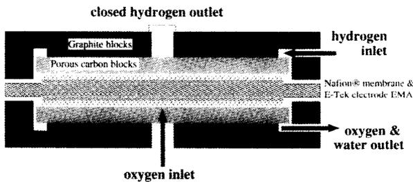
Fig. 2. Schematic drawing of the gas feeding principle in the 100 cm<sup>2</sup> internal hydration PEMFC.
