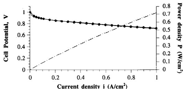
Fig. 5. Fuel cell potential–current density profiles (with power density) for Nafion<sup>®</sup> 112 EMAs with E-TEK ELAT electrodes loaded at 0.35 mg Pt/cm<sup>2</sup> under 4/6 bar pressure of H<sub>2</sub>/O<sub>2</sub>: (○) potential at 80 °C; (●) potential at 100 °C; (–) power density at 80 °C, and (...) power density at 100 °C, lines on the potential points plot Eq. 2 fits.
