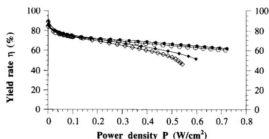
Fig. 6. Plot of the cell total yield rate for different EMAs at two temperatures: (◆) Nafion<sup>®</sup> 117 at 100 °C; (○) Nafion<sup>®</sup> 112 at 80 °C, and (●) Nafion<sup>®</sup> 112 at 100 °C.
