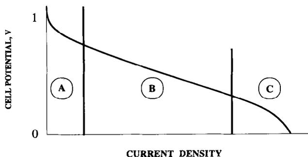
Fig. 1. Typical  $V-i$  profile showing the three zones: (A) activation; (B) ohmic loss, and (C) mass transport limitations.
